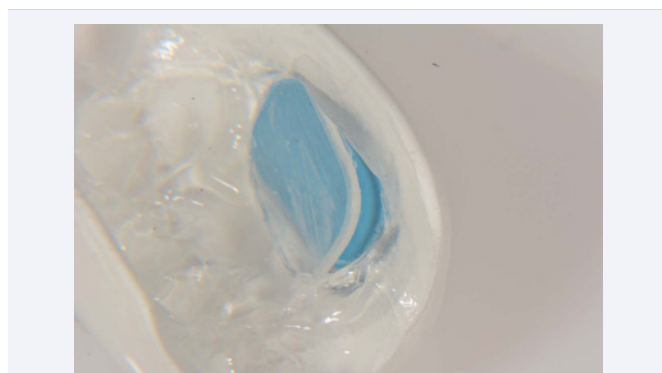
Figure 5 View of the sealing system for the microchip inside the mouth guard.
